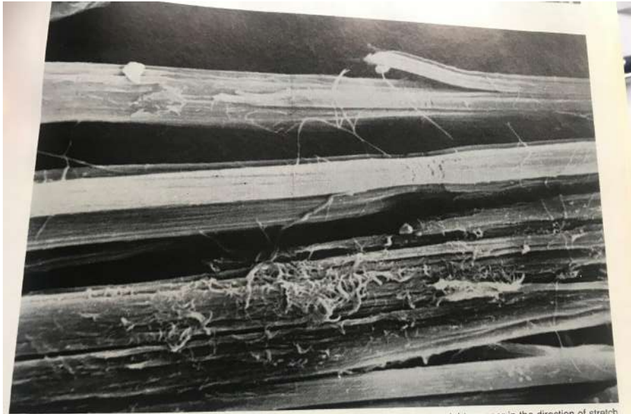
Figure 7-3. When skin is stretched, many of the fibers become aligned in a straight manner in the direction of stretch, thus imposing a limit on extensibility in that direction. (From Brown, I. A.: Structural and Mechanical Studies on Human Skin . Ph.D. Thesis, University of Strathclyde, Glasgow, 1971.)
